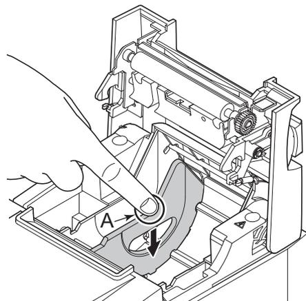
**Note:** After using a paper roll with a width of 57.5 mm, do not change to a paper roll with a width of 79.5 mm. (This is because the printer head has deteriorated as a result of a portion of the head having been in direct contact with the platen.)
